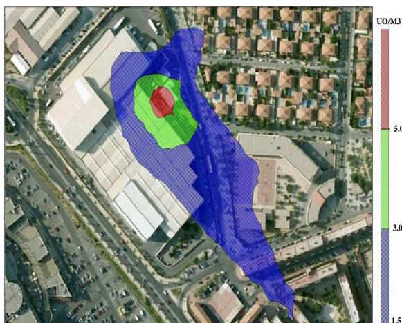
Figure. 3 Results of odor simulation for IWWTPE-EN 13725
